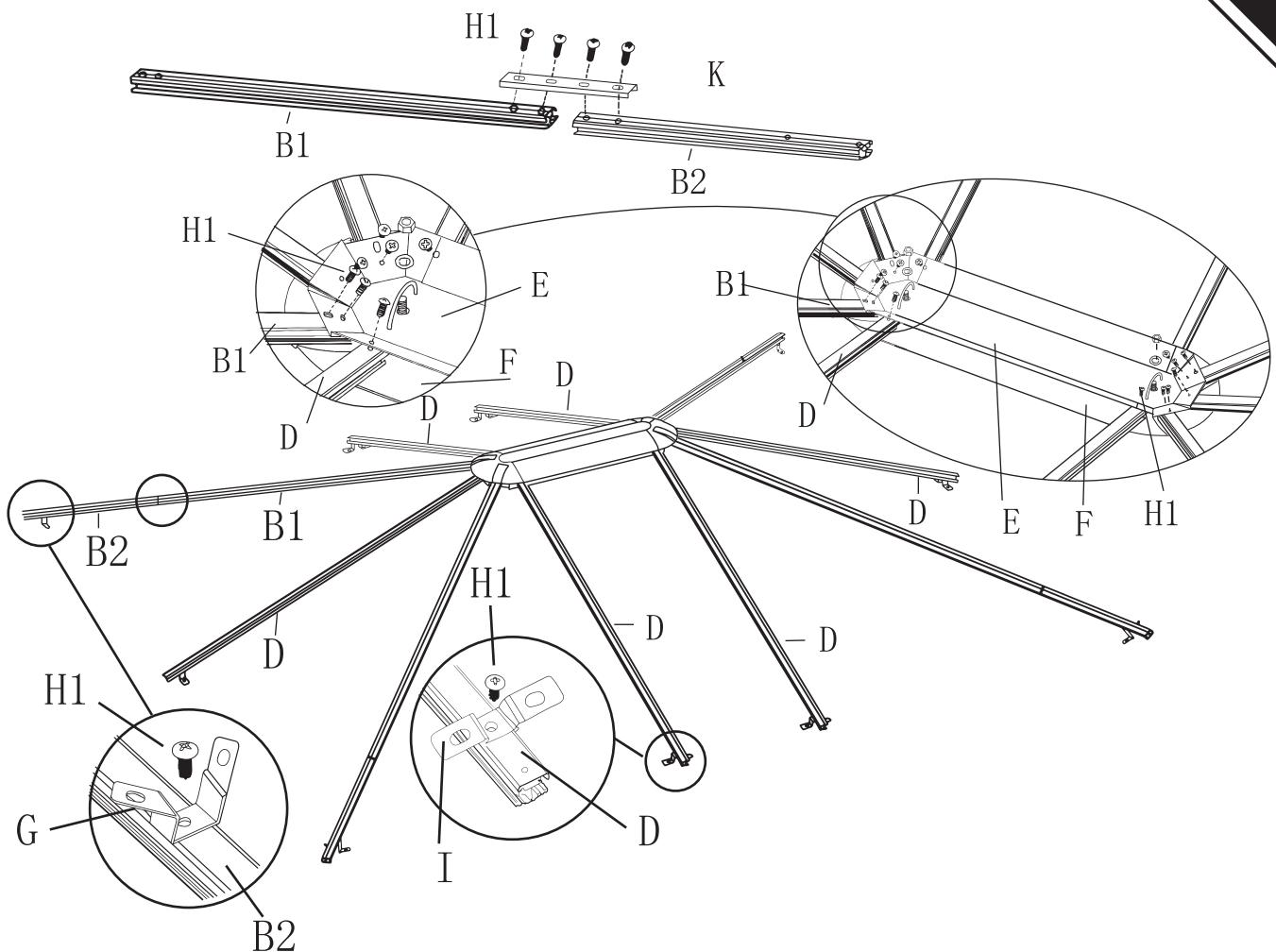
**EN** Note: Before attaching F with E, remove the nut & washer that on the screw of F at first, after assembled, use the nut & washer to tighten the screw.
