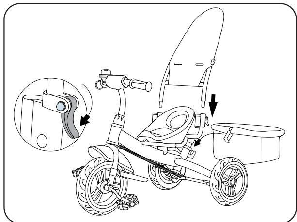
6. As shown in the picture, insert the guardrail bracket into the seat tube and secure it with screws. Then, pass the bolt through the bolt hole indicated by the blue arrow to connect the saddle to the main frame, use a bolt to connect the components in series, and tighten it.
