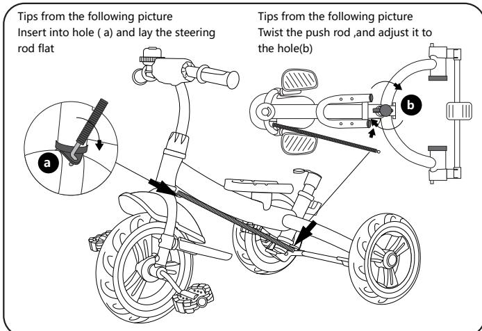
4. As shown in the picture, first insert the front wheel assembly into the main frame, then fit the front cover into the handlebar opening, and then insert the handlebar opening into the fork's upper opening, aligning the fork screw hole with the handle screw hole. Insert the handlebar fixing screw through the opening; then, using a socket wrench, tighten it and lower the front cover. Finally, install the bell on the handlebar.
