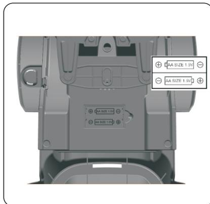
Turn over the tractor body, and find the battery house. Loosen the screw with a screwdriver (not included). Put 2 AA batteries in the battery house, then tight the screw with a screwdriver (not included).
