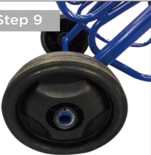
**EN** Step 9: Position wheels (M) onto axle and gently hammer spring clips (N), one each side of reel, onto the axle, clips facing outwards, until wheels are held securely with no lateral movement.
