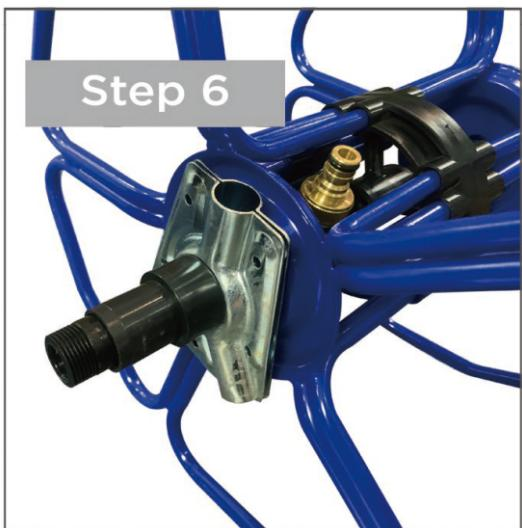
**EN**\_Step 6: Loosely assemble clamps (J) using the M4 bolts & nuts (L) , so that the support frames (B) and axle (C) can slide into them. Position them on the shoulders of the spacers (F).
