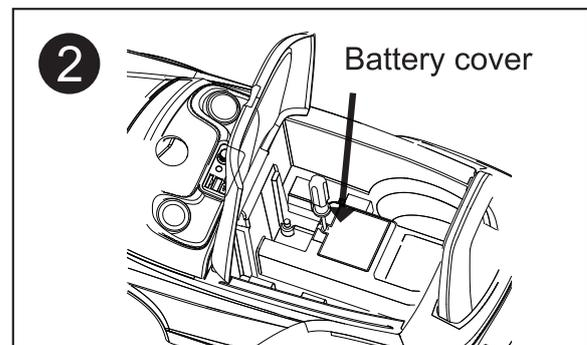
Use a Philip Screwdriver to unscrew the battery cover.
