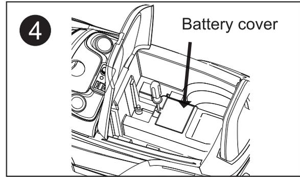
Use a Philip Screwdriver to screw the battery cover.
