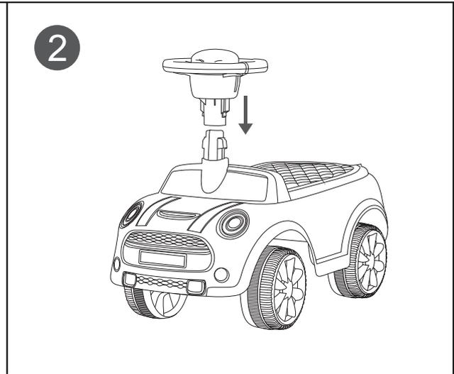
2 Assemble the Steering Wheel with Screw A as shown in the figure.
