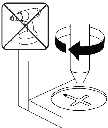
**EN**\_Turn cam lock clockwise to tighten.
