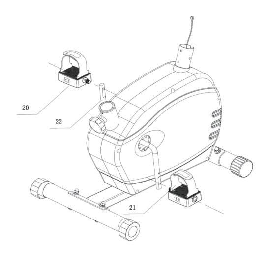
Attaching the pedals to the crank assembly:
