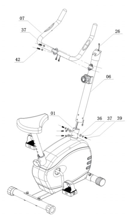
Assembling and fixing the armrest securely:
