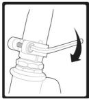
Check and secure all fasteners before every ride. Ensure the collar clamp is locked correctly into position before every ride.
