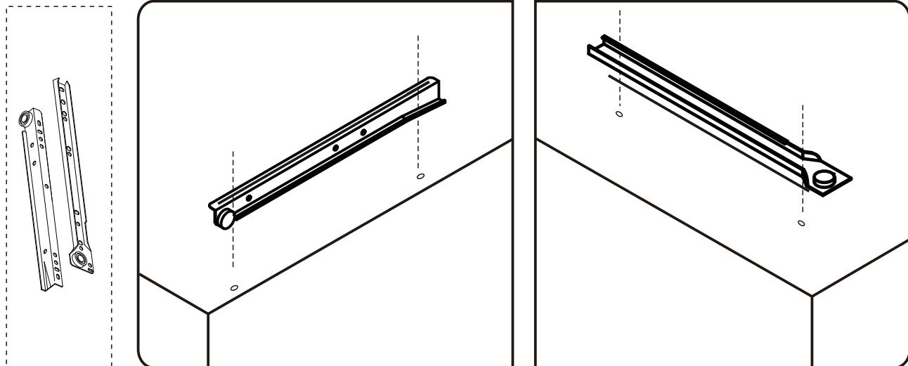
**EN** Please find the exact hole for installation, otherwise it will be misaligned. The screws on the drawer slide must be leveled , otherwise it will affect the smoothness of the d rawer.
