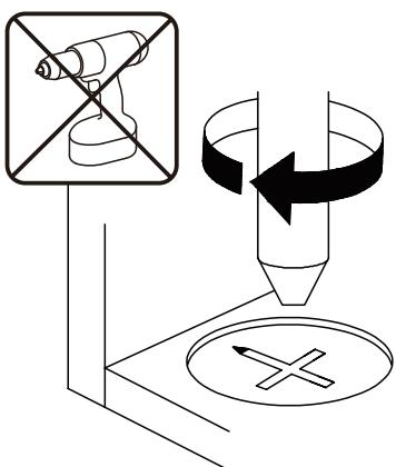
**EN**\_Turn cam lock clockwise to tighten.
