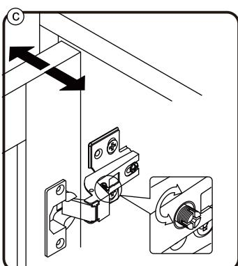
**EN** To adjust the door laterally adjust the screw as shown by turning clockwise or anti-clockwise.
