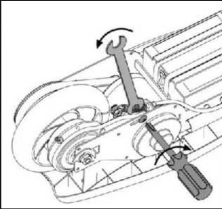
8. Re-tighten the brake arm bolt with a Phillips screwdriver and 8mm wrench.
