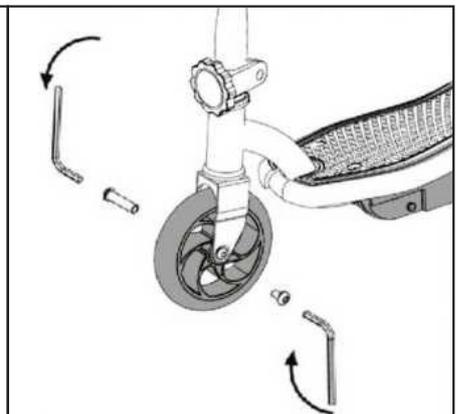
3. Reinstall the parts and tighten with a 5mm hex wrench in a clockwise direction.
