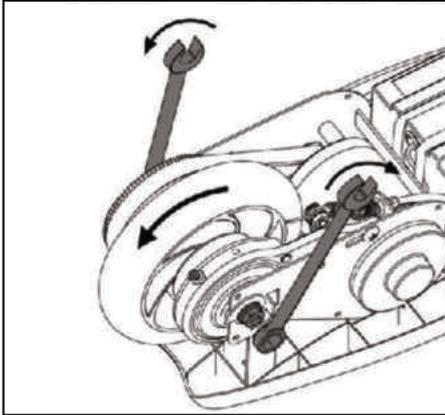
7. Ensure that the adjusting washers are correctly positioned against the frame. After tightening the axle nuts with a 13mm wrench check the alignment of the wheels and the tread of the belt by turning the wheel in the opposite clockwise direction by hand. You may need to adjust the washers to align the belt.
