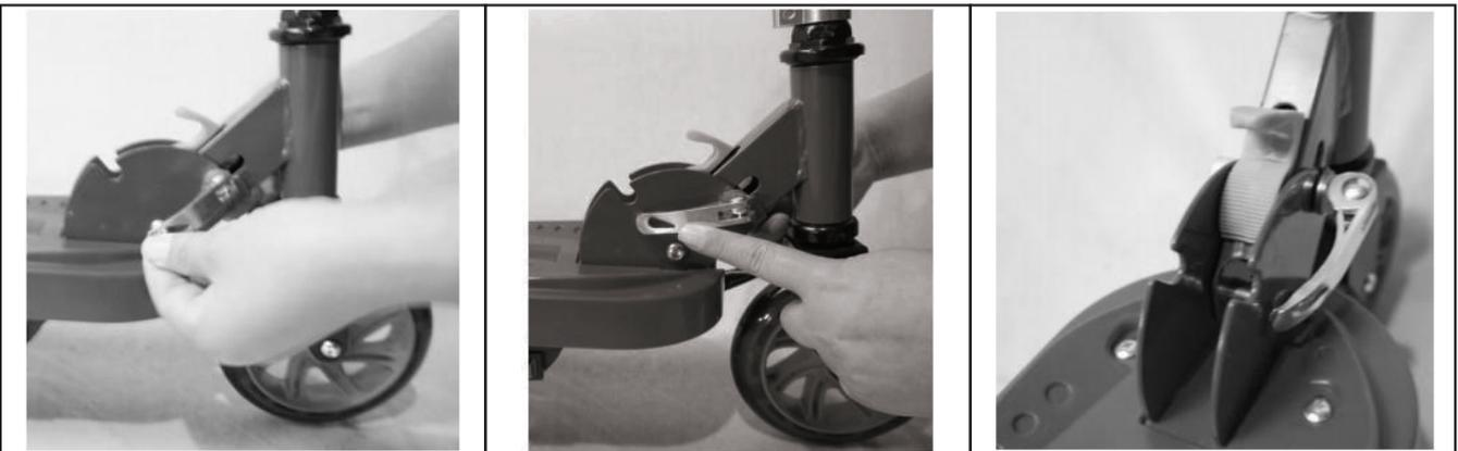
4. Twist the locker of the locking mechanism then tighten it fully and lock it tighten before ride.
