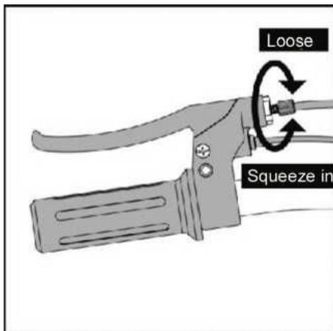
1. To adjust the brake cable wire, turn the adjuster drum on the brake lever clockwise (to loosen) or anti-clockwise (to tighten). Adjust the drum in small increments to the desired setting. If the brake still requires adjustment, proceed to the next step.
