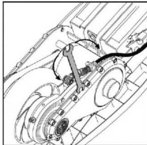
2. If the brake cable is still too tight, use a 10mm wrench to tighten the brake cable for additional adjustment on the cable. Make sure that the 10mm nut is tightened after adjustment.
