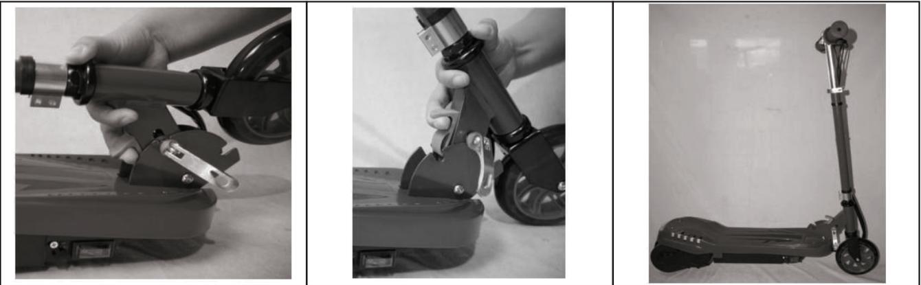
2. Use the finger to lift up the hook of the folding part.
