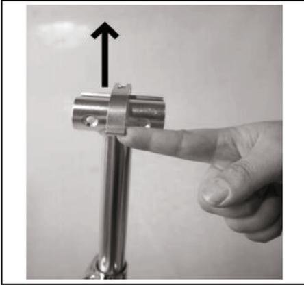
1. Lift up the locker in the T-bar of the handlebar.
