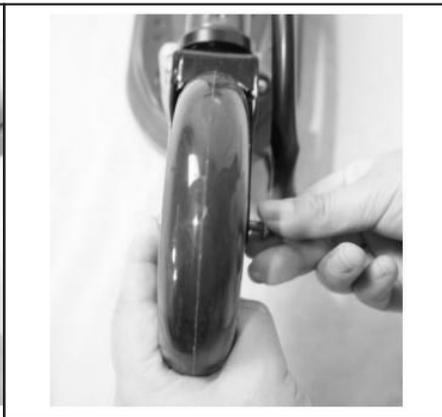
5. Insert the screw of the axle to the hole of the front fork.
