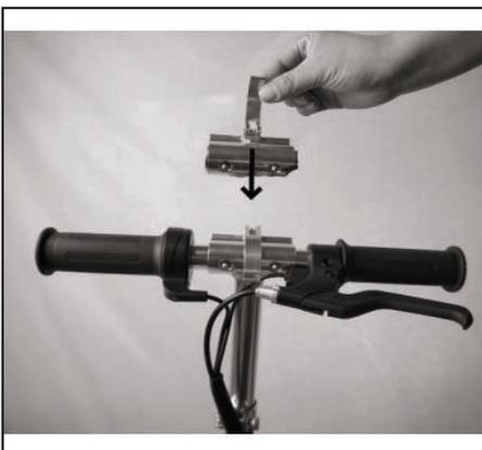
4. Press down and tighten the locker in the T-bar of the handlebar.
