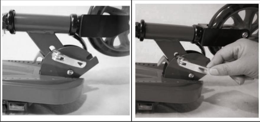
1. Release the locker of the locking mechanism.
