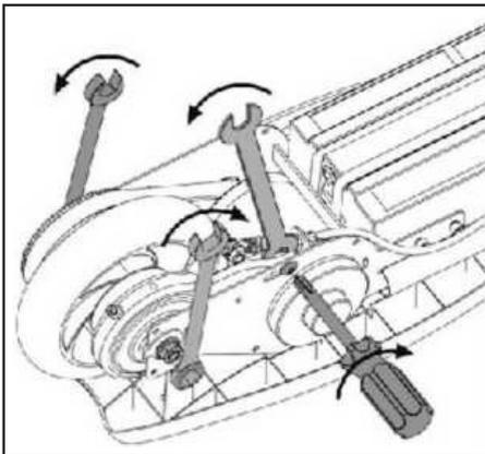
4. Make sure the wheel is aligned in the Frame and tighten the two axle nuts with a 13mm wrench. Re-tighten the brake arm with a Phillips screwdriver and 8mm wrench.
