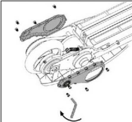
10. Reinstall the side covers with a 4mm Allen key. Do not over tighten the screws.
