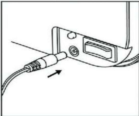
1. Make sure that the switch is in the off position before plugging in the charger. Insert the charger into the charge close on the right side of the battery case.
