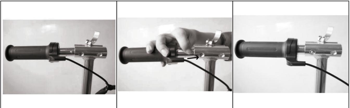
2. Insert the right handlebar of accelerator and use the finger to press the snap pin to insert and fix with the hole in the T-bar of the handlebar.
