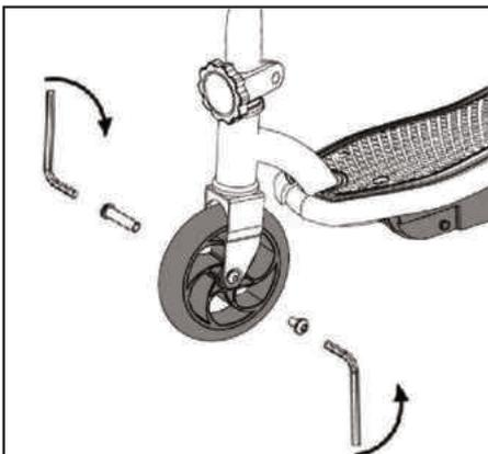
1. Using two 5mm hex Wrenches loosen and remove the front axle by turning the keys to the left.
