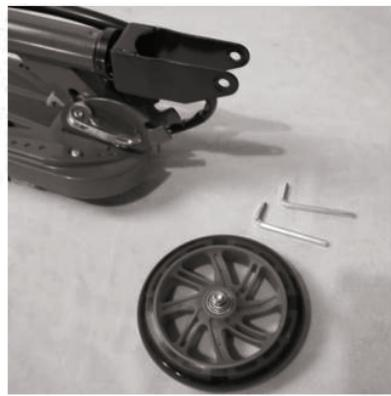
2. Take out the front wheel and the 2\*5mm hex wrench to assemble.
