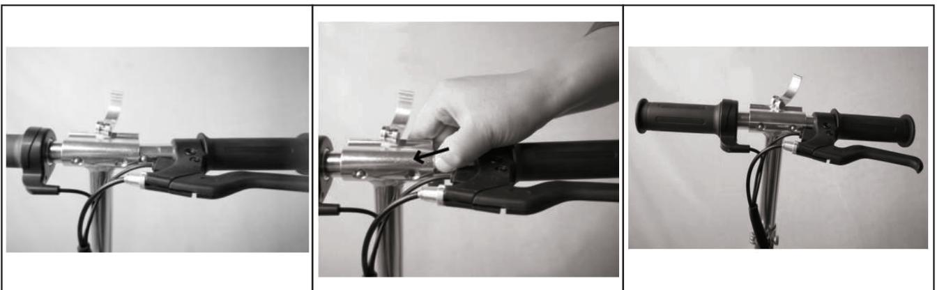
3. Insert the left handlebar of hand brake and use the finger to press the snap pin to insert and fix with the hole in the T-bar of the handlebar.
