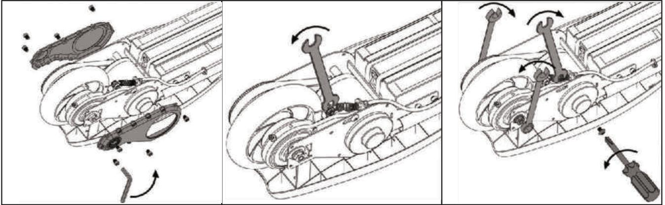
1. Using a 4mm hex wrench, remove the 4 bolts from the rear axle cover on both sides of the scooter. (Only for the scooter with covers.)
