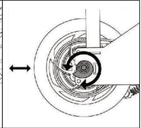
3. Turn the adjusting washers against the frame eyelash to increase or decrease the belt tension. The recommended belt tension is based on being able to bend the belt by approximately 90 degrees.
