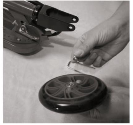
3. Take out the screw of the axle in the front wheel.
