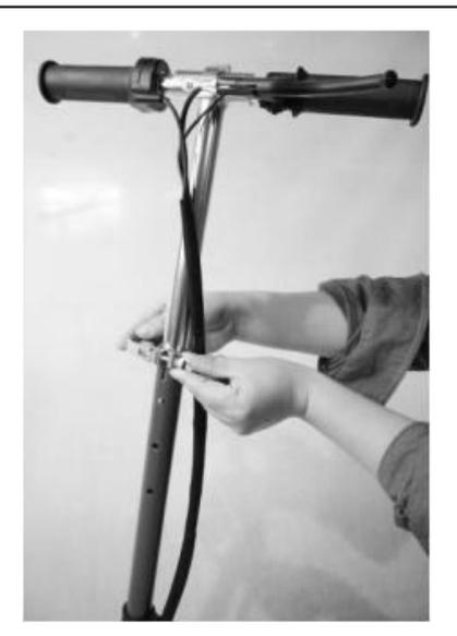
2. Press the snap pin and lift up or down the T-bar to adjust the height.
