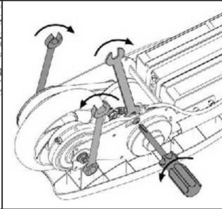
2. Loosen the brake arm with a Phillips screwdriver and 8mm wrench. Using two 13mm wrenches loosen the wheel nuts on the rear axle.
