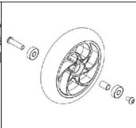
2. Reinstall the spare wheel verifying the order to ensure the location of all components.
