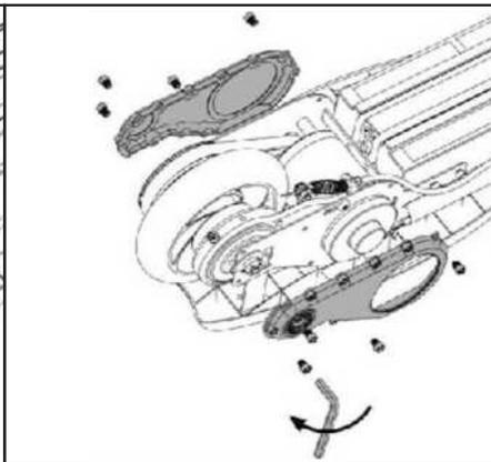
5. Reinstall the side covers with a 4mm Allen key. Do not over-tighten the screws.
