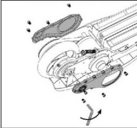
1. With a 4mm hex wrench remove the 3 screws on the protective cover on both sides of the scooter.
