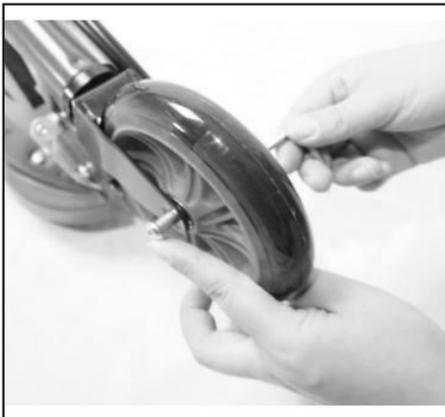
4. Use 1\*5mm hex wrench to lead and insert the axle to the hole of the front fork.
