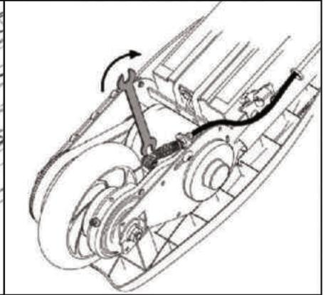
9. Re-tighten the brake cable nut slightly with a 10mm wrench.
