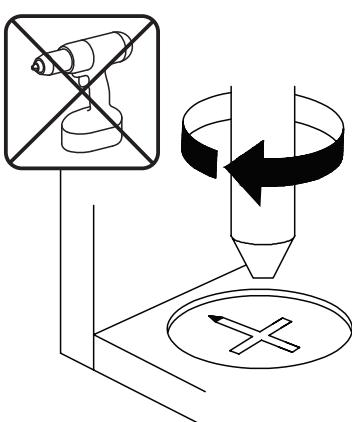
**EN**\_Turn cam lock clockwise to tighten.
