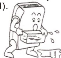
12. Before moving or transporting the machine, pour out the accumulated water in the water tank.
