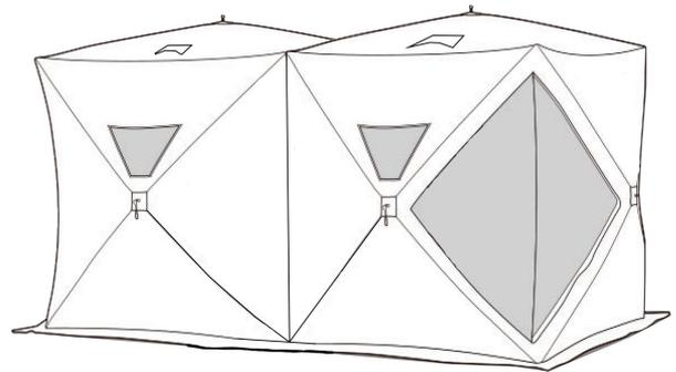
Lifting the roof of shelter up, pull outward on the center hub of one of the walls. Continue around the entire shelter, pulling each wall hub until all of walls are set up.
