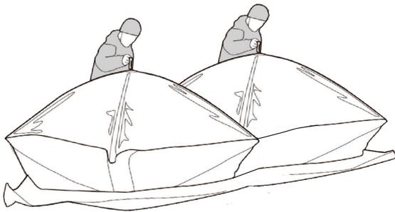
Firmly push down on the the center hub(s) of the roof with the palm of your hand until the roof flattens down onto the sides.
