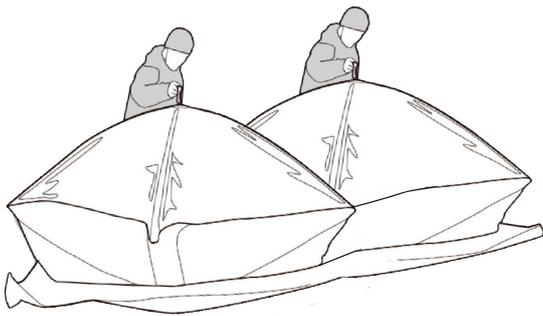
Firmly pull up on the strap in the center hub of the roof until it pops up. Twist the roof slightly so corners of top and bottom line up.
