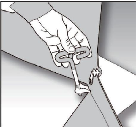
Position the Fish Inn over fishing hole in the ice, and secure each inside corner of shelter to ice by screwing one of the included ice spikes through the 'small loop into ice. Push down while twisting ice spike until it gets started, and then twist the spike until it holds fast.
