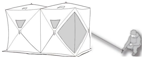
Find the side of the Fish Inn that faces into the wind and attach one of the provided straps to the center hubs of that wall. Stretch the strap into the wind and with the remaining Ice Spike(s), secure the strap to the ice.
