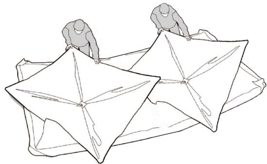
Once the unit is laying flat, lift each of the corners together and stand the folded unit with all of the hubs facing down.
