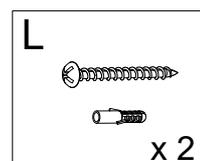
**EN\_ If it is a solid wall, please use expansion and self-tapping screws, if it is a wooden wall, only use self-tapping screws, please do not overtighten the screws**
