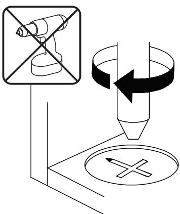
**EN**\_Turn cam lock clockwise to tighten.
