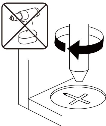
**EN**\_Turn cam lock clockwise to tighten.
