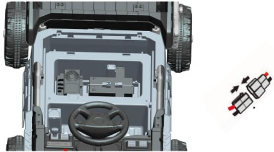
Plug the connector from the battery to the terminal from the vehicle body, match the same color.
