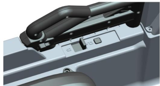
The switch needs to be locked when the scraper bowl is loaded, at the same time the dump bed button on dash board has no function. When you want to unload, you need to unlock the switch.
