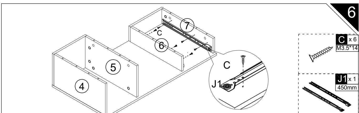
**EN** Please find the exact hole for installation, otherwise it will be misaligned. The screws on the drawer slide must be leveled , otherwise it will affect the smoothness of the d rawer.
