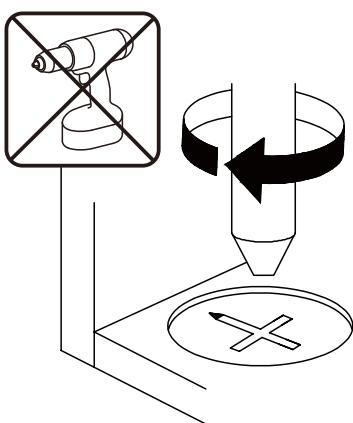
**EN**\_Turn cam lock clockwise to tighten.
