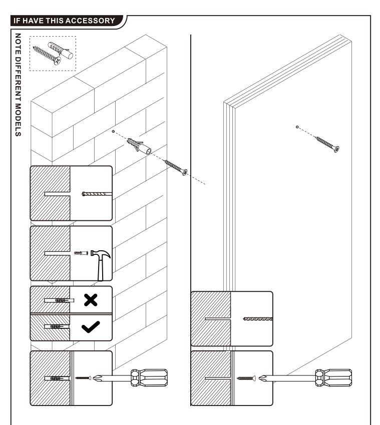
**EN\_**If it is a solid wall, please use expansion and self-tapping screws, if it is a wooden wall, only use self-tapping screws, please do not overtighten the screws
