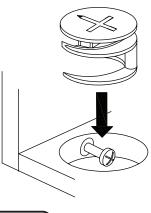
**EN\_Quickfit** head should be in the centre of the cam lock when the two panels are joined.
