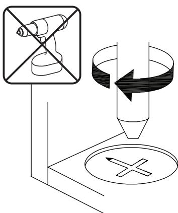
**EN**\_Turn cam lock clockwise to tighten.
