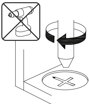
**EN**\_Turn cam lock clockwise to tighten.
