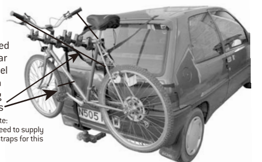
Fitting cycle frame straps
