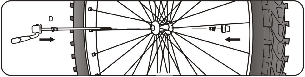
Use quick release bolt(D) to align the axle of the bicycle.
