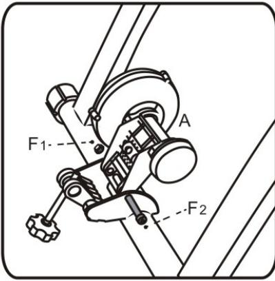
Insert the screw(F2) into the main machine(A), tighten the nut (F1) with the tools(G,H).
