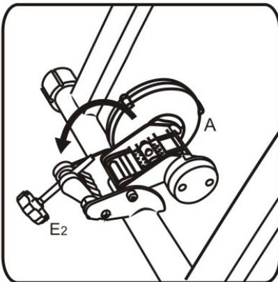
Turn machine(A) to another side, let knob scrow(E2) insert to the circular groove on main machine(A).
