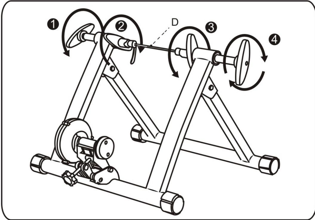
Tighten wheel with this 4 knobs(#1,#2,#3,#4)with correct direction as shown in image.
