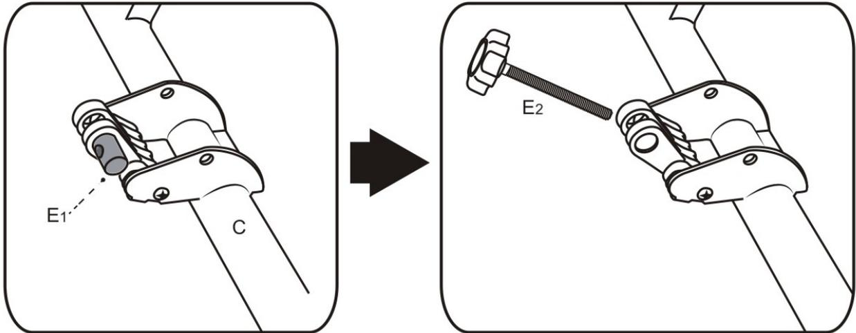
Put (E1) into the sleeve of main frame(C) , then twirl screw(E2) into the sleeve.
