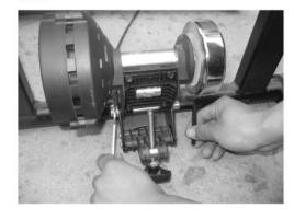
4 To change the height of magnetic wheel by adjusting the knob after assembling the magnetic so as to fit different sizes of bikes.
