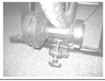
The bike trainer can be adjusted to fit wheel sizes from 66cm to 700C (69cm). Turn the adjustment knob (H) so that the wheel is touching the bike trainer.
