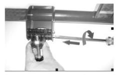
3. To fasten the magnetic wheels withthe given tools
