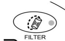
**FILTER Key** - On-off key for the filtration system. Press this key, and the filter pump will start working and the red indicator lamp will be on. Press again the pump will stop working and the lamp will be off.
