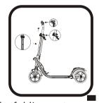
Pull the plastic hook upwards to unlock the folding system and pull the handle bar stem downwards. When you sound clicks, the scooter is completely unfolded.
