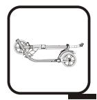
Loosen the quick lock, press the spring button and push down the T-bar at lowest height level. Then tighten the quick lock to secure the T-bar.
