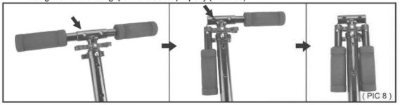
$Loosen\ quick\ lock,\ press\ spring\ handle\ and\ push\ downwards\ to\ lowest\ lever\ and\ then\ tighten\ the\ quick\ lock.$
