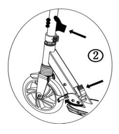
Release quick lock. Pull upward and adjust T-bar to three right height position according to user height.
