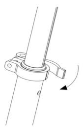
Pull apart handle grip from grip bracket and press the handle into T-bar. Ensure the spring handle pops out to secure in position properly.
