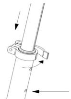
Press spring handle and pull outwards handle grips. Hold on grips on grips bracket.
