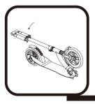
Loosen the upper lock, press the spring button and push down the T-bar to the lowest height.
