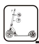
Push the folding button and pull up the handlebar until it clicks. Release the handle from the grip bracket and insert it into the T-bar, ensuring the spring button pops to secure it into it position.
