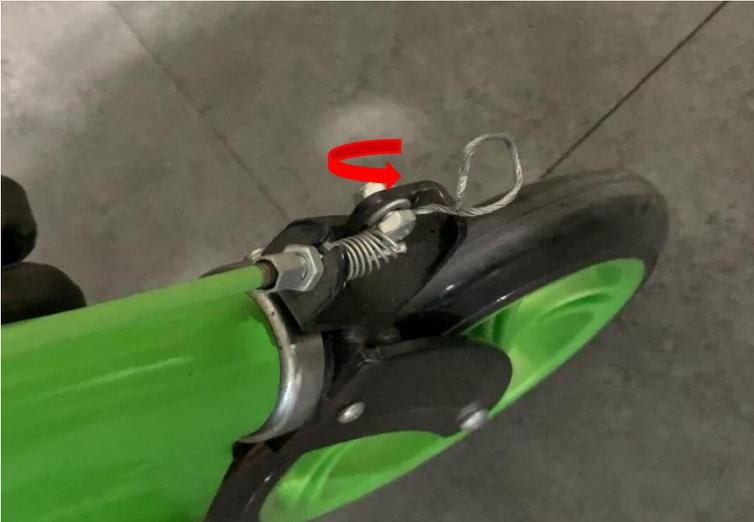
2. Tighten the brake rope while screwing the nut.
