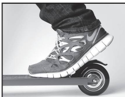
With the heel of that foot, **GRADUALLY** apply pressure to the top of the brake mechanism. This will decrease your speed and eventually bring you to a stop.
