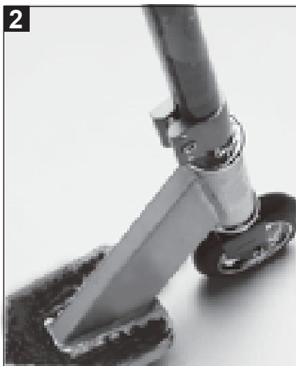
Adjust the **Front Wheel** and the **Clamp** so that the **Front Wheel** is perpendicular to the **T-Bar**.
