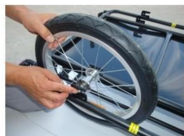
A. put the wheel into the frame as picture
