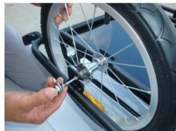
B. insert the quick release into the wheel axle
