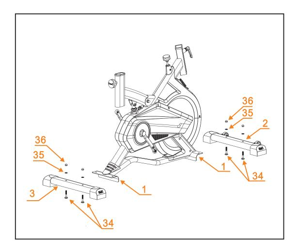
AS THE PICTURE SHOW, INSERT THE 4 CARRIGE SCREW (34) TO FRONT AND REAR STABILIZER, TOGETHER WITH THE FRAM (2/3). PUT THE GASKET IN IT (35), AND FIX IT WITH NUT BOLT (36).
