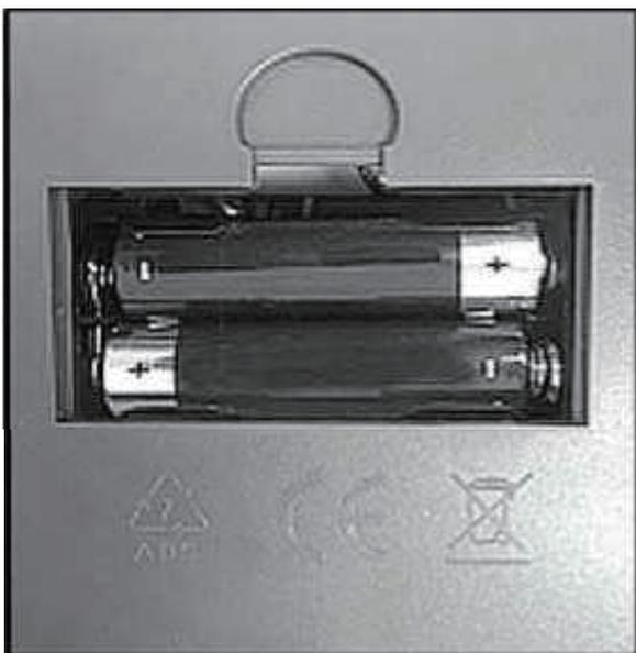
3. Install 2 AA batteries according to the correct polarity.
