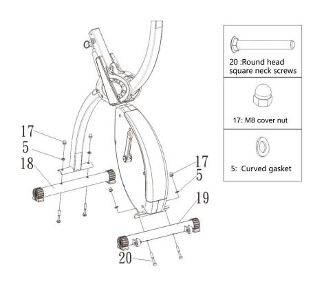
Step two: assemble the tripod
