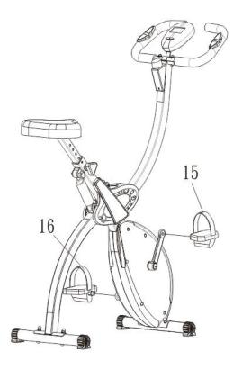
Step 6.Assemble the foot pedal
