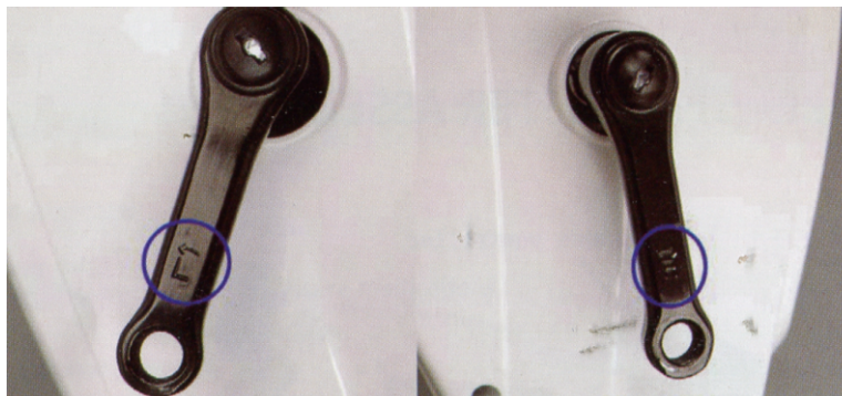
left pedal arm Screw the left pedal into the left pedal arm counter-clockwise
