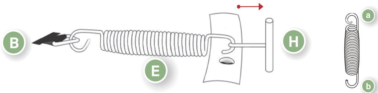
6. Hold Spring Tool (H) overhand and pull spring hook towards Top rail (c) as picture shown: drop hook into frame hole until it latches on completely, tap it down if hook is not completely in the hole.
