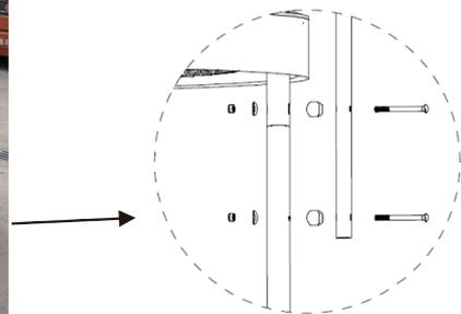
A1: Mount the upper poles onto the vertical leg extension using parts of spacer, washer, screw, and nut.
