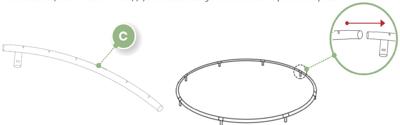
3. Two people will be necessary at this point to assemble the trampoline. One person lifts up the circle frames. The other person lifts the W shaped leg tubes to a standing (vertical) position and inserts the T-connectors into a U shaped leg tubes. Ensure the locking holes are aligned.
