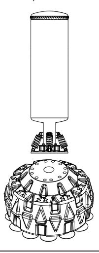
5.Connect the sandbag to the base with 12 screws, and tighten them one by one with an installation wrench.
