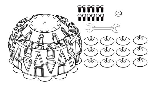
2.Take out 12 suction cups, turn the bottom of the bucket up, align the screws with the holes below the base, and tighten them one by one
