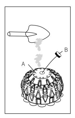
4. After installing 12 suction cups, Next take out the 12 screws placed on the cylindrical base and fasten the two, as shown in the figure below.
