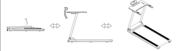
Screw off T shape and flower shape knob to fold the machine. Fix the two kinds of knobs to set up machine.
