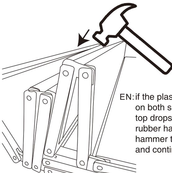
EN: if the plastic connectors on both sides of the table top drops, you can use a rubber hammer or wooden hammer to knock it back in and continue to use it.
