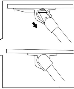
EN: Fix the frame with table top as shown in picture. Please pay attention to keeping the hole on frame corresponded to the bulge under the table top.
