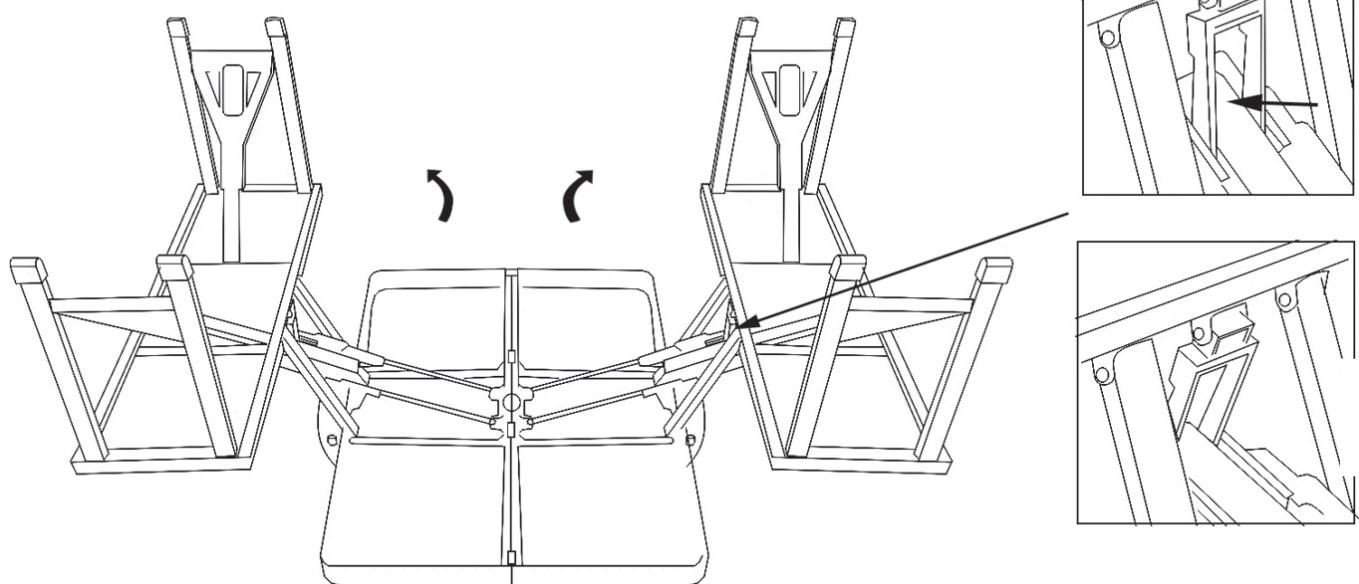
**EN** Push the safety lever to end as shown in picture
