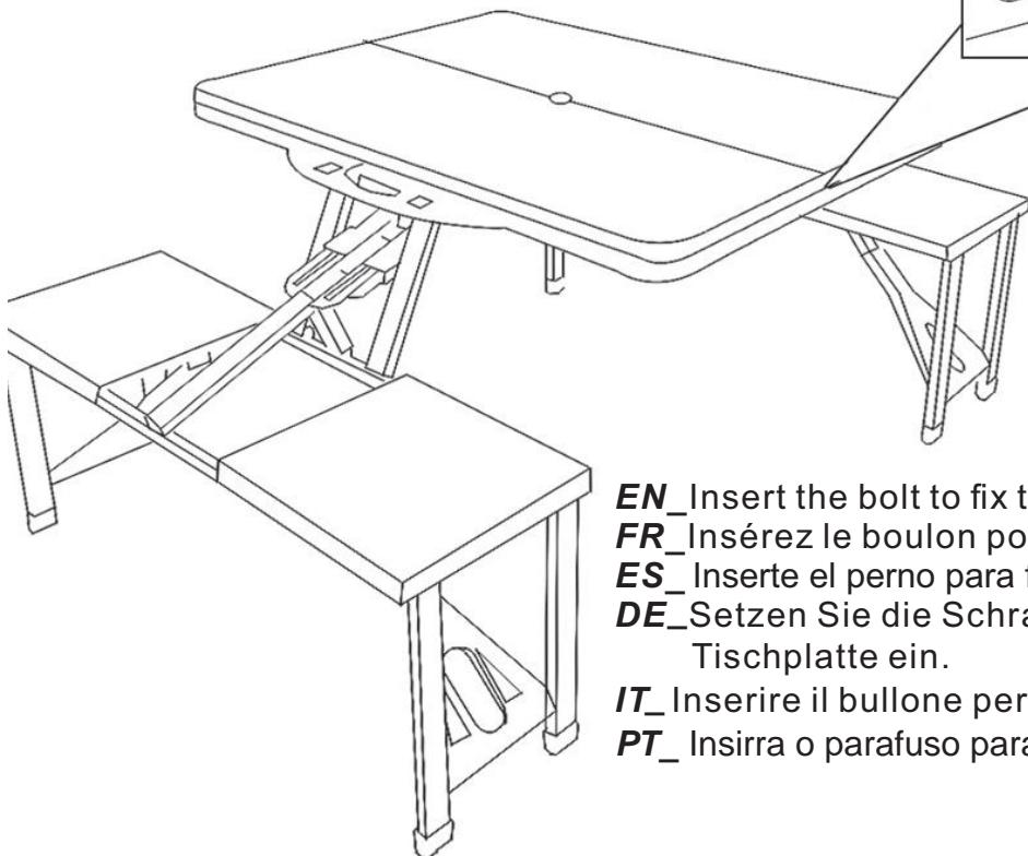
**EN**\_Insert the bolt to fix the table top
