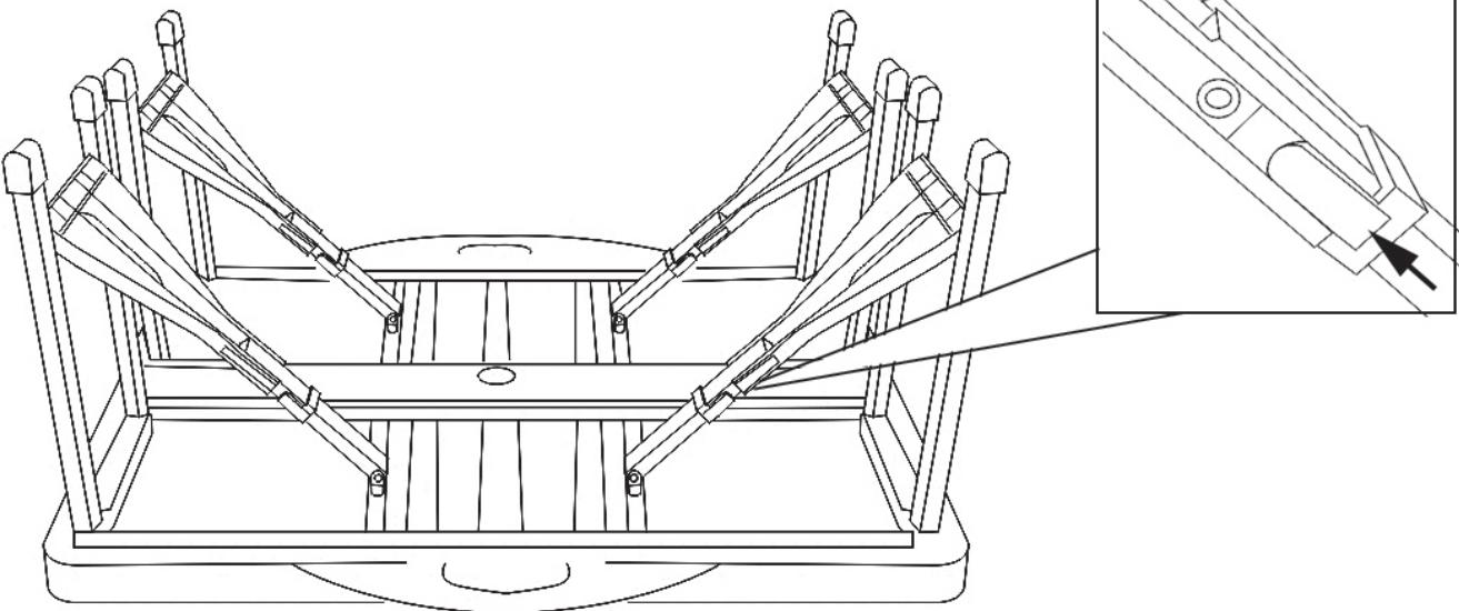
**EN** Pull out leg frames and push the plastic buckle to lock it as shown.
