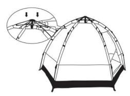
3. Hold the top of the automatic tent pole, lift it up, so that the hexagon of the tent is naturally unfolded, put down the tent, make sure that the hexagons are supported on the ground, then press the middle post to the hands as shown, after having heard the "click", the tent was initially installed.
