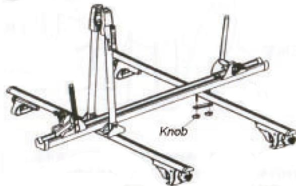
**5** Open the locking device with key
