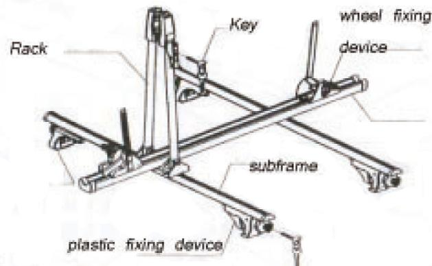
**2** remove the fixing plate at the bottom of rack
