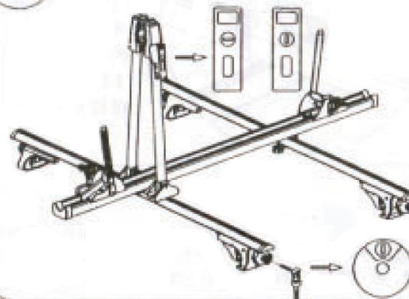
**6** Place the assembled bike rack to the roof of car and set the position. Lock the plastic fixing device
