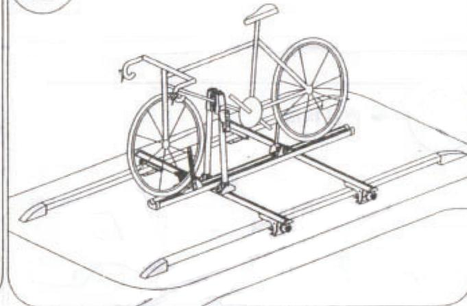
**10** You can set the position of wheels fixing device according to the bike type
