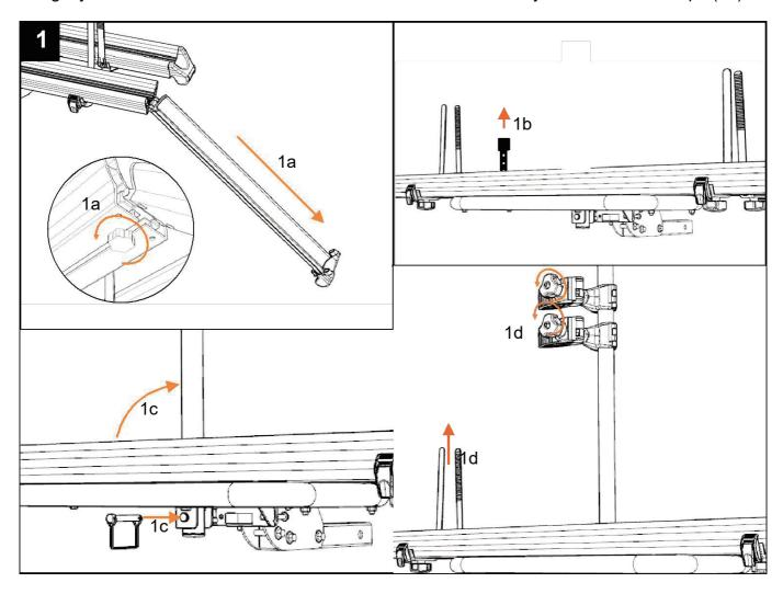
**Note:** You can roll your e-bikes onto the trays from either the left or the right by unscrewing the screws under the trays, then lifting and reversing the whole trays.
