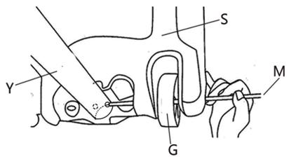
Insert the Wheel Shaft (M) into Wheel(G), Base(S) and end of Bottom Pole (Y) as shown.
