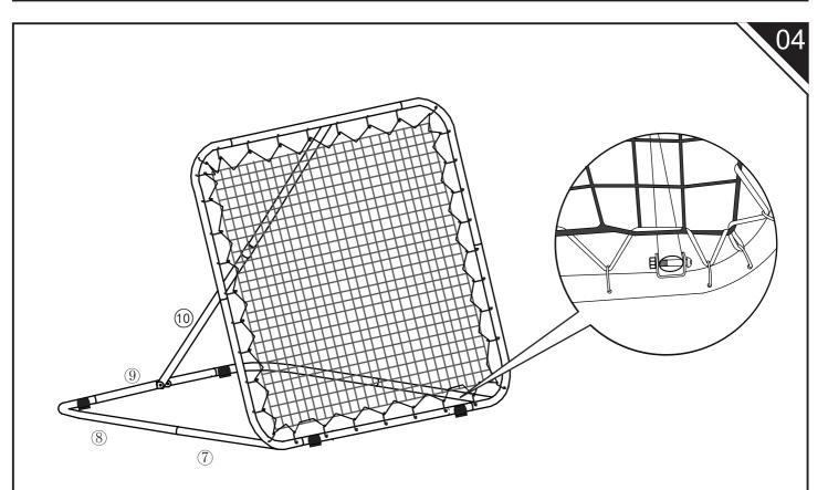
**Tips:** To avoid the metal plate part when assemble the net on the frame.
