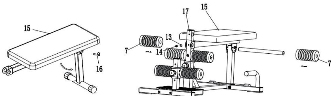
STEP 5: Part 15 out of box, Rotate to 90° (as photo show). Then fix by Pin (part 16). Put Part 15 and standing (part 17) together according Part 6. There are 3 holes can be choosed.
