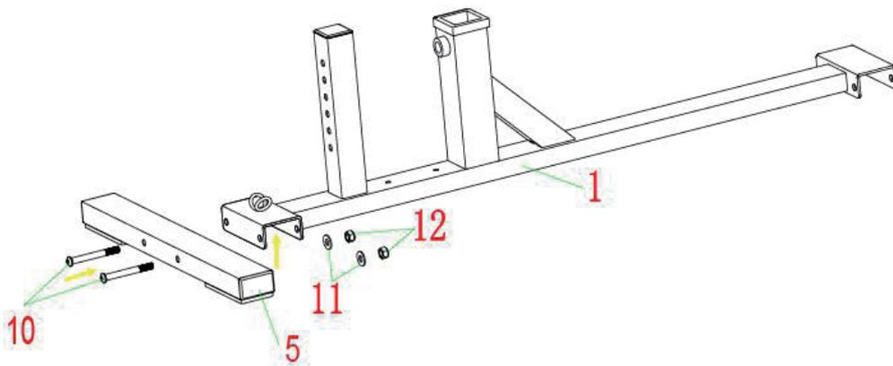
STEP 1: put the part 1 and part 5 out of carton and lay them on ground. Put the part 1 and part 5 assemble together by Part 10, 11, 12
