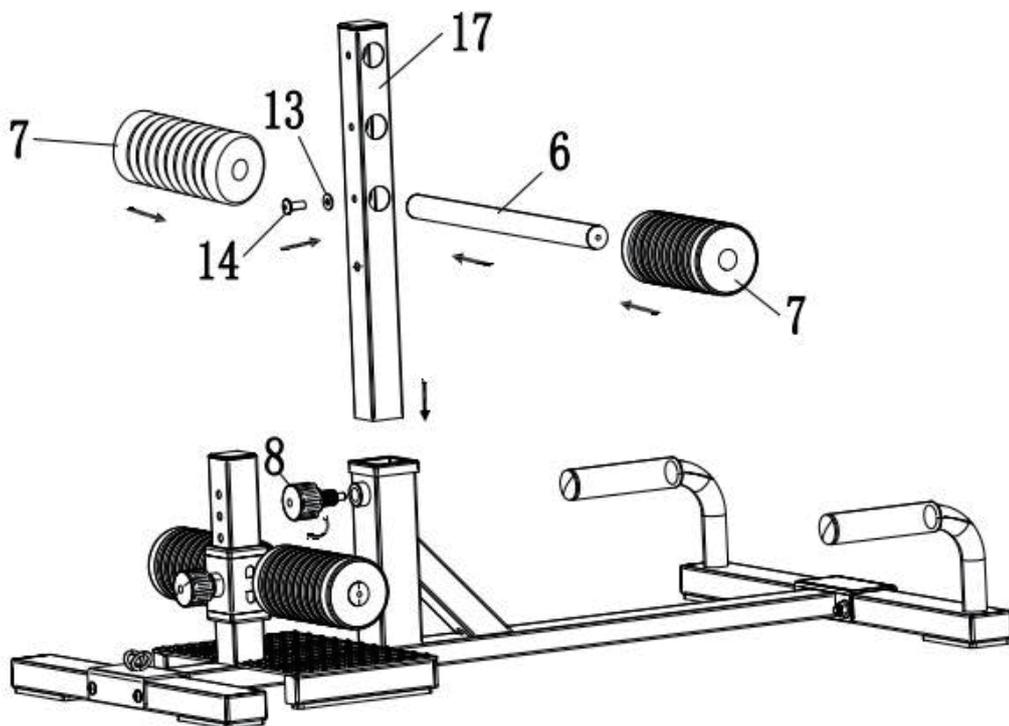
STEP 5: Install Poam 7 into Part 6 and Part 17, And fixed part 6 by screw (part 14)
