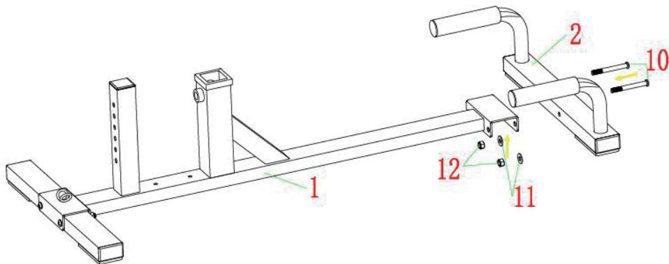
STEP 2: put the part 1 and part 2 out of carton and lay them on ground. Put the part 1 and part 2 assemble together by Part 10, 11, 12
