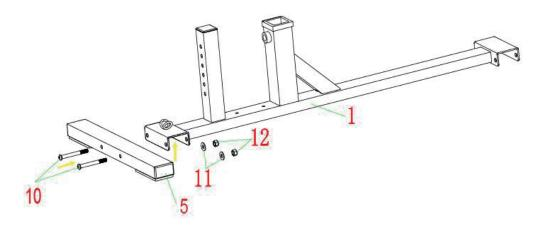
STEP 1:put the part 1 and part 5 out of carton and lay them on ground. Put the part 1 and part 5 assemble together by Part 10, 11,12
