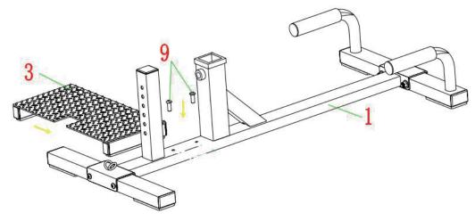
STEP 3:Put the part 3 and part 1 assemble together by Part 9
