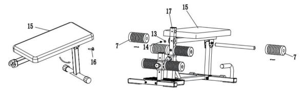
STEP 5:Part 15 out of box,Rotate to 90° (as photo show) .Then fix by Pin(part 16) Put Part 15 and standing (part 17) together according Part 6.There are 3 holes can be choosed.
