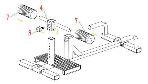
STEP 4:Install Poam 7 into Part 4,Then install Knob 8 into standing,You can adjust the height according to Knob 8.
