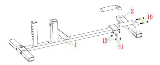
STEP 2:put the part 1 and part 2 out of carton and lay them on ground. Put the part 1 and part 2 assemble together by Part 10,11,12
