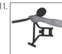
11. Assemble the handle by placing the structure (6) on the bars (7) with two washers (38) and two nuts (34)
