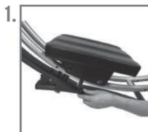
1. Attach the seat to the bow-rail using the side bolt.
