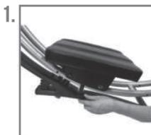
1. Attach the carriage to the blow-rail using the side bolt.
