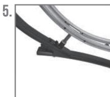
5. Insert the bow-rail (4) into the main structure using one screw (24 M8x15) and one washer (40).
