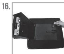
16. Screw the cushion (9) to the carriage table (8) using four screws (24) and four washers (37).
