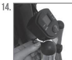
14. Install the computer (10) into the bow-rail support (4) – connect the cables.
