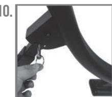
10. Insert the large safety bolt (A) to set the desired SLOPE.
